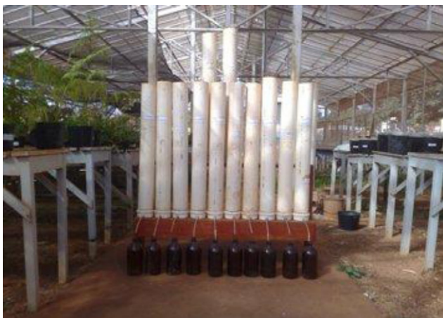
Fig. 3. Partial photograph of the P and K leaching experiment.
